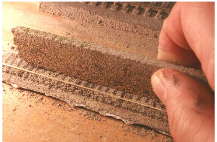
Using scrap cork roadbed to even the ballast with the tops of the ties.
