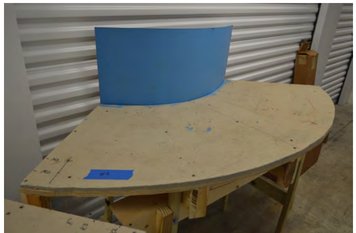
The unfinished modules include backdrops. Track support is 3/4" plywood with 1/2" homosote on top.
